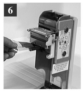
Pull about 6" of dye film off the roll of dye film, observing that it should be coming off the top of the roll, as per the label illustrations.
